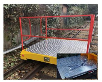
With the addition of bespoke and standard railings the MEP can be turned into an "Emergency Response Vehicle" The umbilical controller now clips to the railings where ever the nominated driver is standing. The unit can be used by emergency responders in full protection suits and BA equipment to get them to site of emergency quickly. The deck comes with evac chair and stretcher securing systems as an option.
