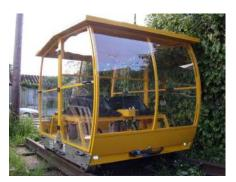
Various roof options are available whether it's a canopy to keep the sun out, roll down pvc windows for hostile weather or full enclosed cabin for DCL can manufacture a bespoke system. All units are removable and foldable for easy storage and transportation
